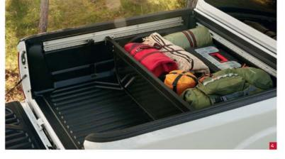
1- Tool box plastic <sup>(65)</sup> 2- Sliding tray<sup>(61)</sup> 3- Retractable rear step <sup>(67)</sup> 4- Bed divider <sup>(66)</sup>
